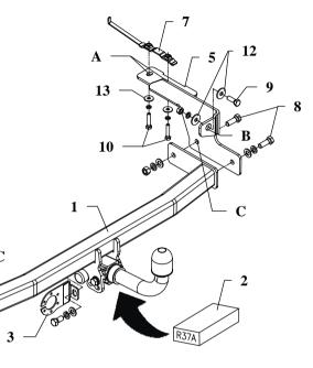
This towing hitch is designed to assembly in following cars: **FIAT IDEA** produced since 2003, catalogue no. **R37A** and is prepared to tow trailers max total weight **1100 kg** and max vertical load **60 kg**.
