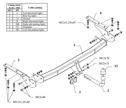
This towbar is designed to assembly in following cars: **TOYOTA RAV-4, model with the spare wheel,** produced since 2009 till 12.2012, catalogue no. **O75** and is prepared to tow trailers max total weight **2000 kg** and max vertical load **75 kg**.
