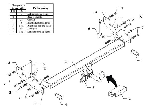
This towing hitch is designed to assembly in following cars: **TOYOTA HILUX 2WD, small wheels,** produced since 2005, catalogue no. **O69A** and is prepared to tow trailers max total weight **2500 kg** and max vertical mass **100 kg**.
