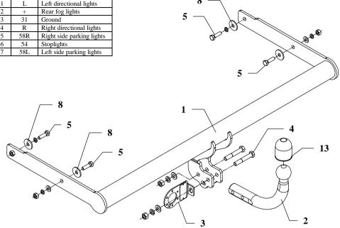
The towbar can be used following in the car: VOLKSWAGEN GOLF III ESTATE, produced since 1993 till 1998, catalogue number K16 and is prepared to tow trailers max total weight 1500 kg and max vertical load 75 kg.
