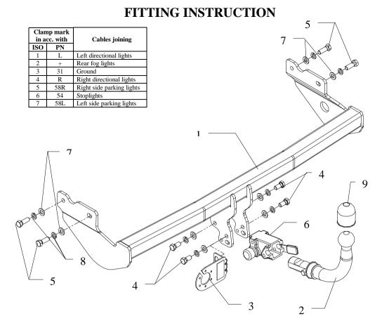
This towing hitch is designed to assembly in following car: **HYUNDAI GETZ**, produced since 2003 till 12.2004, catalogue number **J46A** and is prepared to tow trailers max total weight **1100 kg** and max vertical load **50 kg**.
