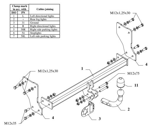
This towbar is designed to assembly in following cars: **HYUNDAI ATOS**, produced since 1998, catalogue no. **J13** and is prepared to tow trailers max total weight **700 kg** and max vertical load **50 kg**.
