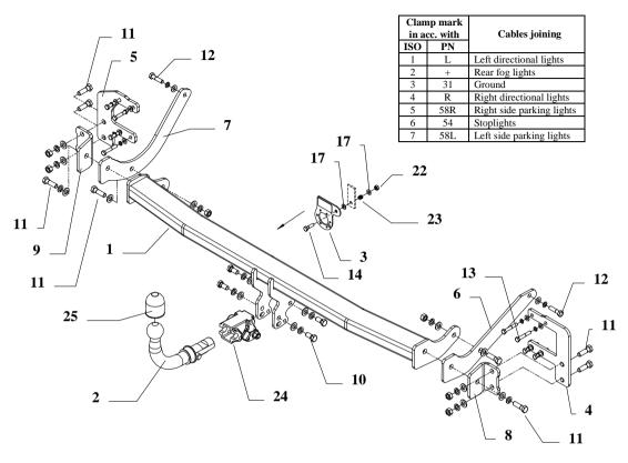
This towbar is designed to assembly in following car: **PEUGEOT 407 4 door,** produced since 2004 till 08.2008 (**Attention! Not suitable for car with 3.0 HDi V6 engine!**), catalogue number **F29A** and is prepared to tow trailers max total weight **1900 kg** and max vertical load **65 kg**.
