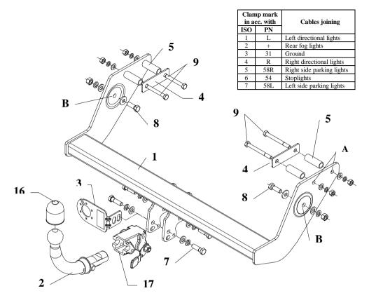
This towing hitch is designed to assembly in following cars: **MERCEDES VANEO** produced since 2002, catalogue no. **D27A** and is prepared to tow trailers max total weight **1200 kg** and max vertical load **50 kg**.
