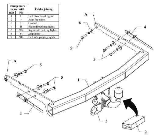
This towing hitch is designed to assembly in following car: **FORD MONDEO, 5 door,** produced since 03.2007, catalogue no. **C54A** and is prepared to tow trailers max total weight **2120 kg** and max vertical mass **80 kg**.
