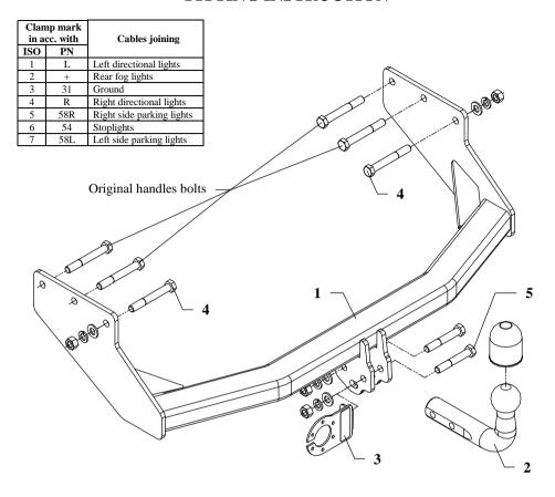
This towing hitch is designed to assembly in following cars: **FORD TRANSIT, metal build-up, loading platform,** produced since 11.1991 till 04.2000, catalogue no. **C18** and is prepared to tow trailers max total weight **2000 kg** and max vertical mass **75 kg**.
