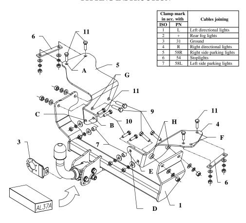
This towbar is designed to assembly in following cars: **ALFA ROMEO 147, 3/5 doors**, produced since 2000, catalogue no. **AL37A** and is prepared to tow trailers max total weight **1300 kg** and max vertical load **60 kg**.
